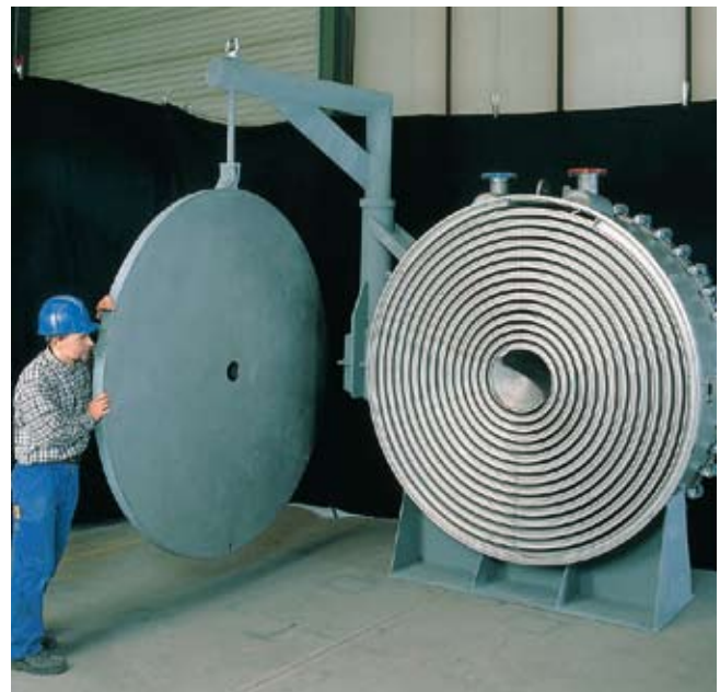
40 m 2 , ø 1900 mm, Sludge Application
