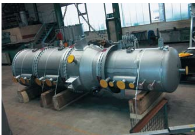
3-stages overhead condenser
