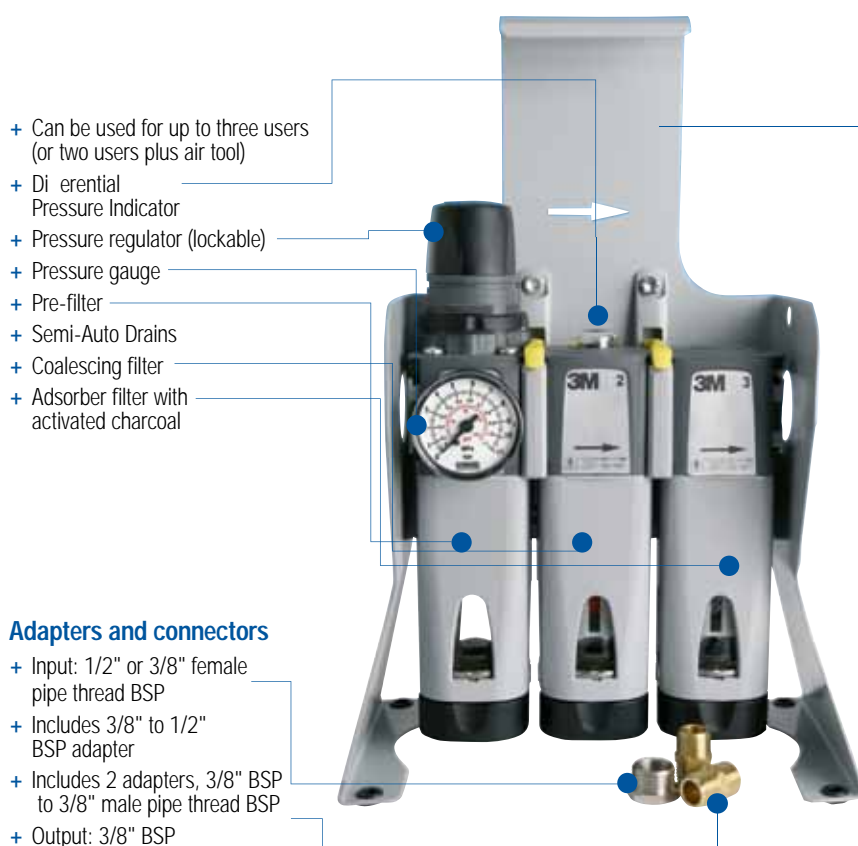
3M™ Aircare™ Filtration Unit ACU-02, Freestanding Input: 1/2" or 3/8" female pipe thread BSP Output: 3/8" BSP
