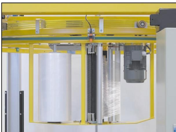
*The Power Pre Stretch film carriage feeds the film evenly with a pre-stretch factor up to 300 %. Stepless adjustable secondary stretching ensures optimum wrapping of a wide range of products.*
