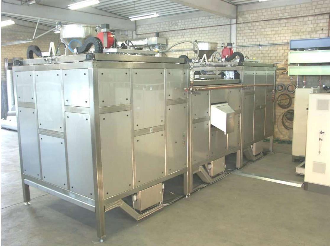
If the roasting time is longer than 6 minutes, two roasters could work at full capacity with a single cooler. This leads to a further reduction of the space required.
