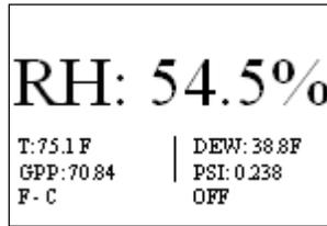
4. **The meter will begin taking readings.** As a default setting the RH reading will be the most prominent on the screen. If you would like to make another variable (temperature, GPP/GPK, PSI/KPA or dew point) the prominent reading, use the  $\uparrow$   $\downarrow$  and  $\leftarrow$   $\rightarrow$  keys to highlight your selection. Press the **SELECT** key to choose that variable.
