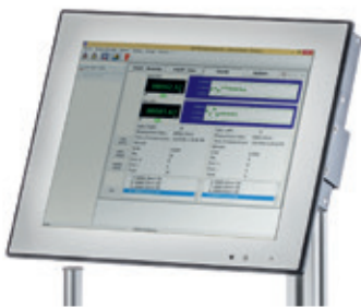
Telso®QS Measuring and process control software Industrial Panel PC 15" touch screen
