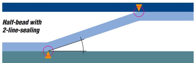
**Half-bead with 2-line-sealing**
