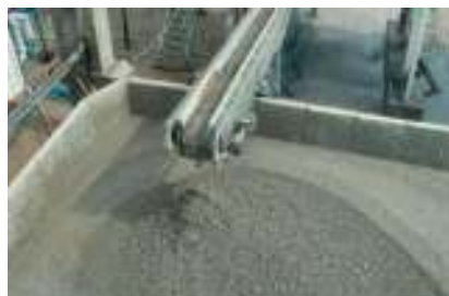
Solids discharge after processing with a Flottweg Decanter
