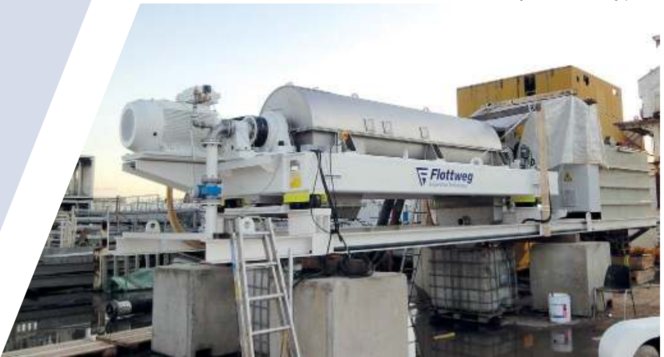
Flottweg Decanter used for drilling operations
