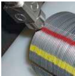
Multi-colored marking of spring rings
