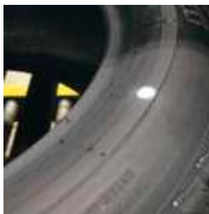
High-point marking on automobile tires
