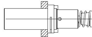
Install with 4 machine screws
