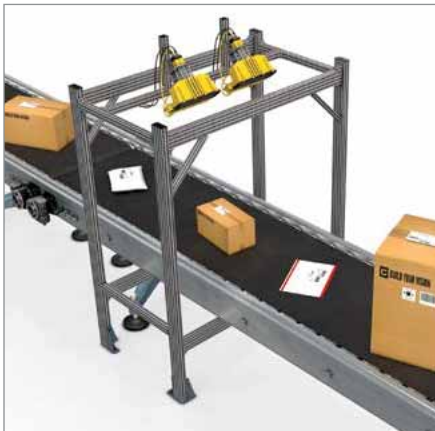
Single-sided scan tunnel
