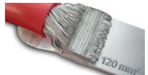
Aluminium wire 120 mm 2 to aluminium busbar
