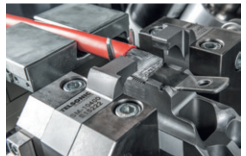
Robust downholder system with cable clamping
