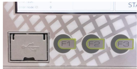
USB connector, freely programmable keys
