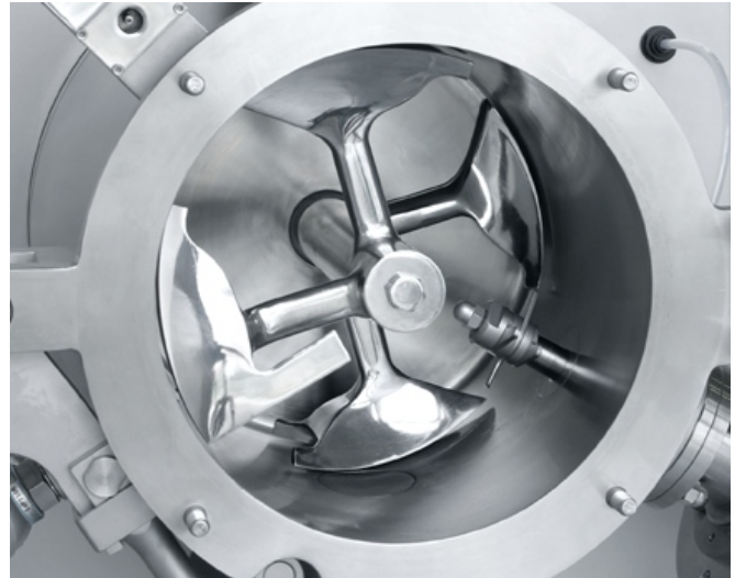
View into the mixing drum
