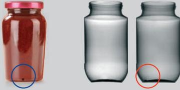
The dual-beam X-ray inspection system prevents blind areas when inspecting jars.
