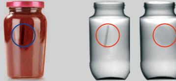
Reliable detection of a thin glass sliver, most likely not detected with a single-beam system.
